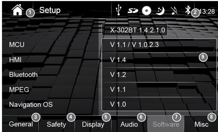
This screen informs you about installed Software versions. Navigation SW is only available at model X-302BT.
